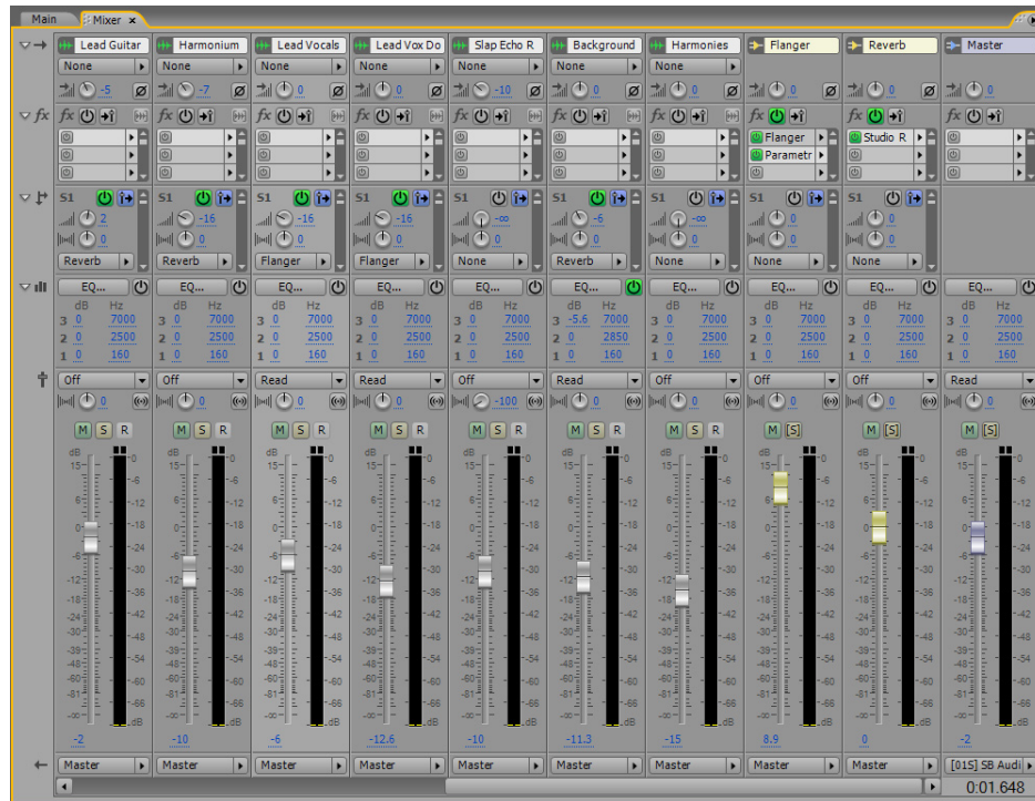
Mixer panel showing several tracks and buses. The Mixer panel shows all of the settings at a glance, including pan and level settings, which effects are applied, and where the track or bus is routed.
